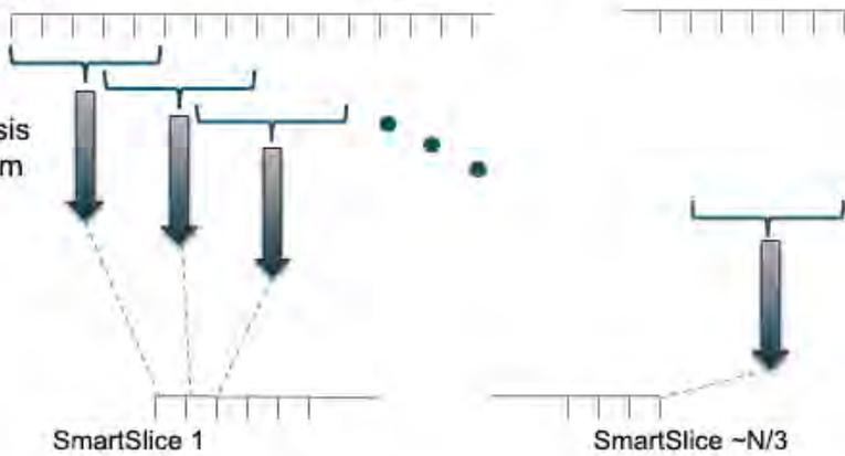
Each SmartSlice is a combination of 6 1-mm slices, with 3-mm overlap from adjacent SmartSlices
